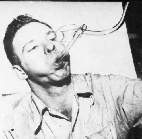
The blower now starts puffing a hot, pliable bit of glass into a pretzel-like curlicue in the sign.
